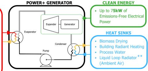
+ Heat Sources that are not water or glycol mixture will require an interface heat exchanger and hot water loop ++Standard Liquid Loop Radiator supplied by ElectraTherm will have a 20°F (11°C) approach to the ambient air
