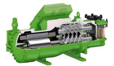
The ElectraTherm ORC design incorporates a BITZER semi-hermetic twin screw expander. Both the expander and generator are integrated within the same housing, eliminating the need for a shaft seal and enhancing reliability. Additionally, the expander is designed for dual-phase flow, allowing for a robust range of operating conditions.
