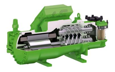
The ElectraTherm ORC design incorporates a BITZER semi-hermetic twin screw expander. Both the expander and generator are integrated within the same housing, eliminating the need for a shaft seal and enhancing reliability. Additionally, the expander is designed for dual-phase flow, allowing for a robust range of operating conditions.
